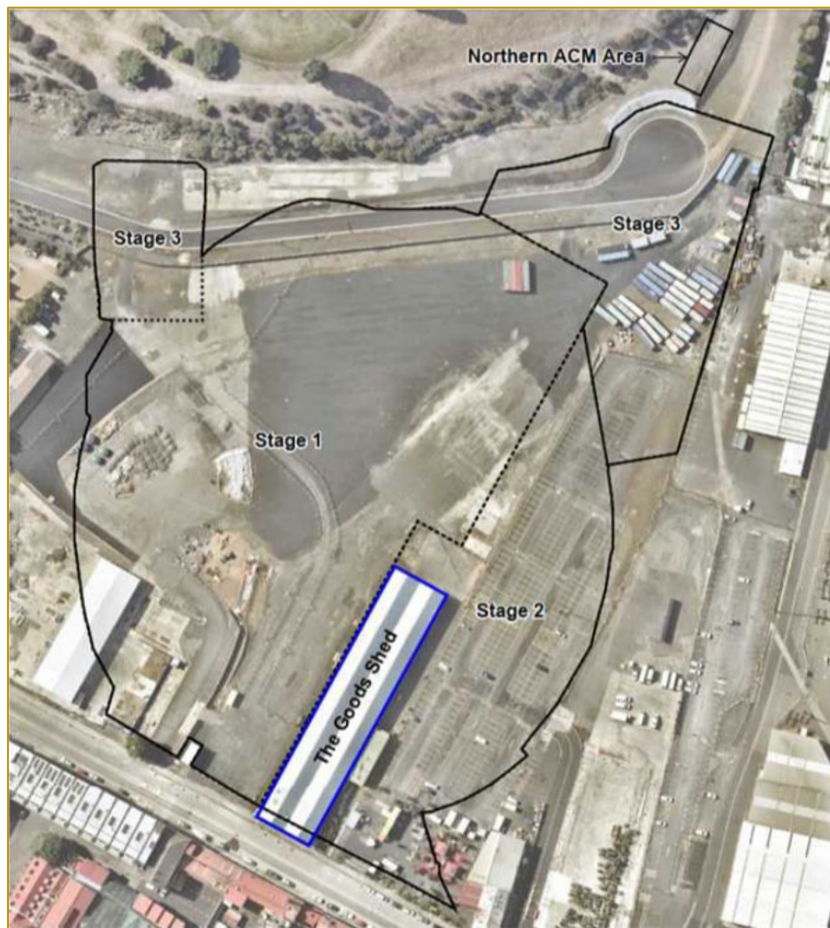
Figure 10: Proposed bulk excavation stages in the future works. Source: Appendix A – Technical Specification: AECOM Bulk Excavation for Future Development (Stage 1 and Stage 2) document accessed 2026.
